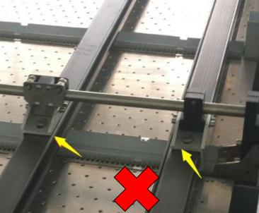
Other company design (Make holes in the guide rail, Damage to the rail body, Inconvenient for maintenance and replacement)
