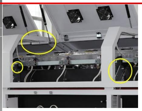
No hole on chamber body design separa tes heat from coming out, ensures m ore accurate temperature performanc e, meantime, machine cover stay cool, low request on air conditioner, electricity energy saving for users..
