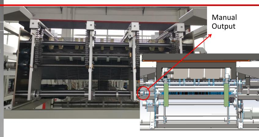
In extreme cases, the PCB on the mesh and guide rail can be manually moved out.
