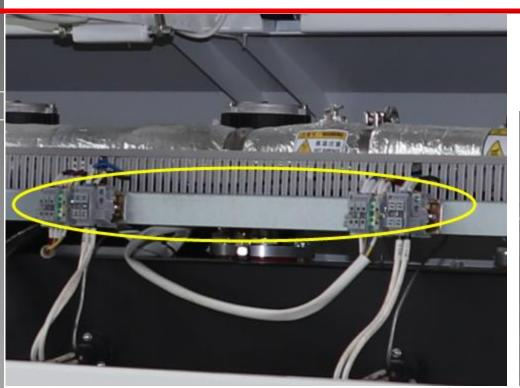
ETA oven all electrical parts and connection points are suspended, not in contact with the oven body, high safety.
