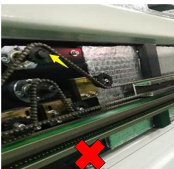
Other company design (Chain drive, poor synchronization, inconsistent width, easy to jam PCB)
