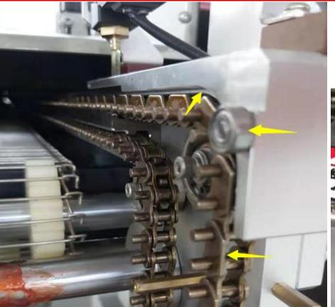
The guide bearing and 4mm chain edg e are special desined to prevent pcb from being blocked.
