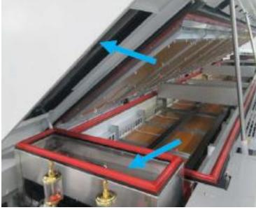
ETA exhaust moves forward, and the open preheat zone has reserved nitrogen buffer zone, which is manufactured as nitrogen machine standard
