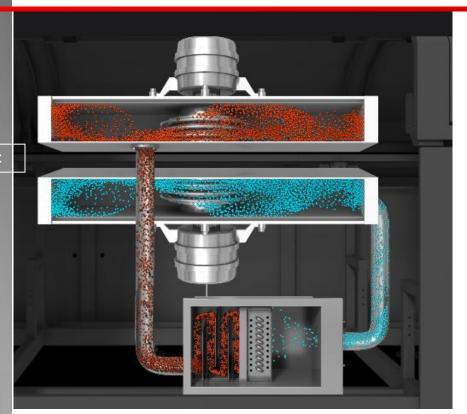
ETA flux management system can effectively manage residue and reduce nitrogen consumption
