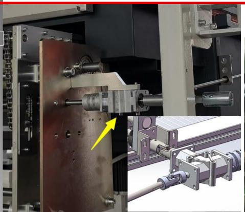
The commutator adjusts rail width, Reliable structure, High synchronization, will not cause the rail to be out of synchronize.
